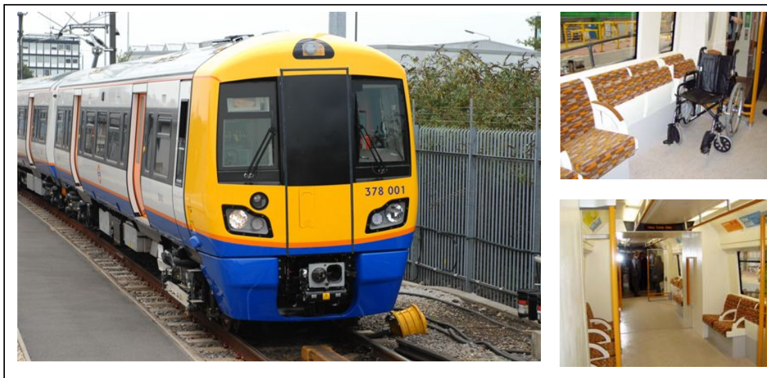
Figure 2: Class 378 Rolling Stock – Both AC and DC variants exist for different traction power systems on the LO network and the interior is designed for high capacity and accessibility
