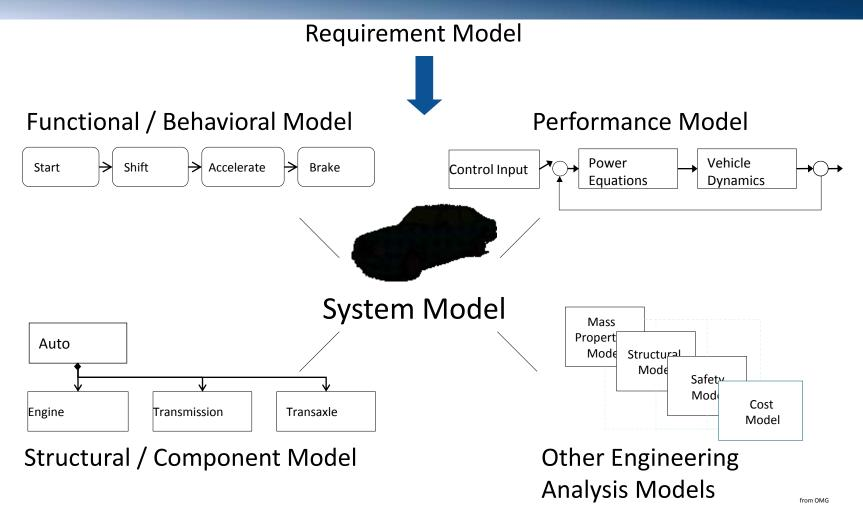
Integrated System Model Must Address Multiple Aspects of a System
