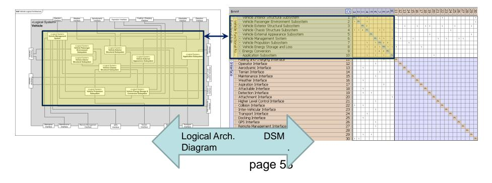
Logical Architecture Views Block Diagram and Design Structure Matrix (DSM)
