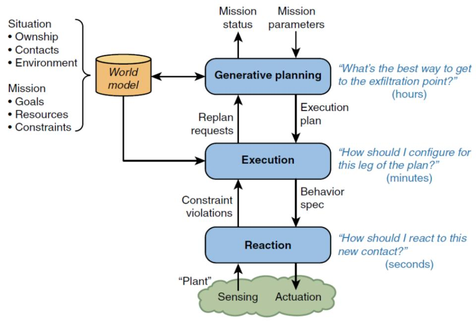
Figure 1. Layered Autonomy Model (Watson & Scheidt, 2005)
