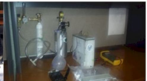
CooRS benchtop prototype for CO 2 removal and O 2 generation. Future uses are foreseen in space, aviation, undersea, and mining operations
