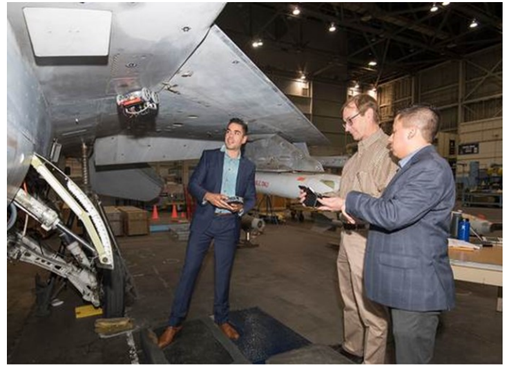
The new Crawler is capable of moving along inverted surfaces as it inspects, because of a suction fan sub-system.
