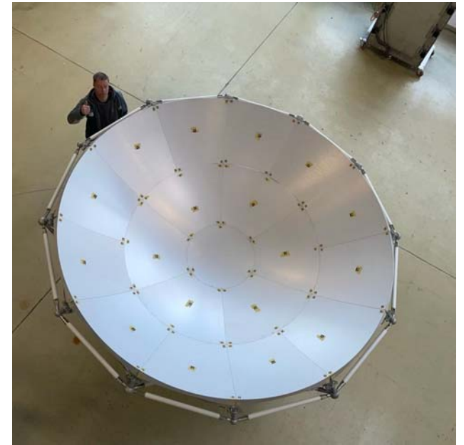
Sub reflector was adjusted with photogrammetry to <30 \mu\text{m RMS}
