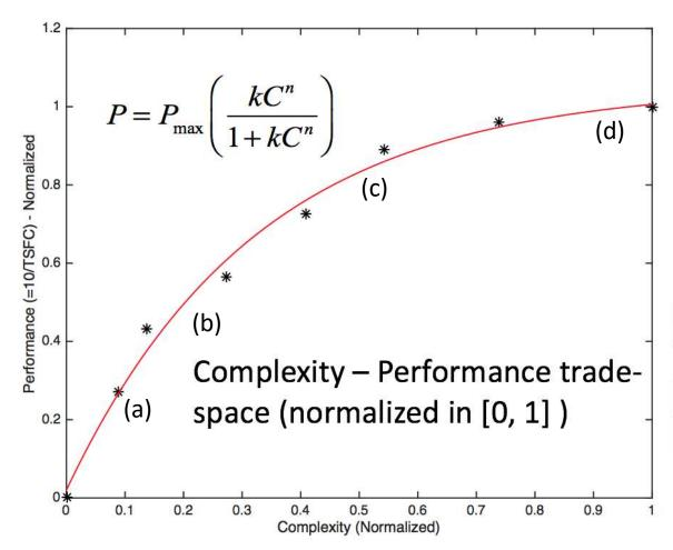
Left: Diminishing returns of normalized TSFC performance for air-breathing aircraft engines versus complexity, Bottom: evolution from turbojet to geared high BPR turbofans
