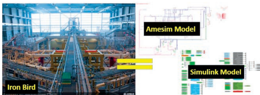
Figure 4. Actual iron bird versus virtual iron bird
