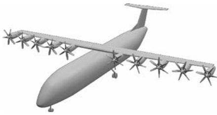
Figure 11. Hydrogen-powered concept aircraft – ESBEF-CP1 (Kuelper et al. 2022)
