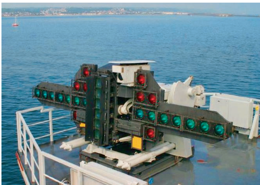
Figure 8. A deck approach light projector mounted on a naval vessel (Burrowes and Squair 1999) (photo courtesy of www.netmarine.net under creative commons https://commons.wikimedia.org/wiki/File:FS_CdG_Optics.jpg )
