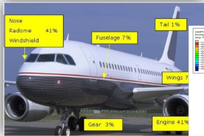
Statistical distribution of impact damage
