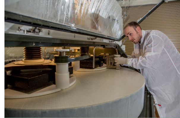
Modular add-on assemblies for ultrasonication and pad conditioning
