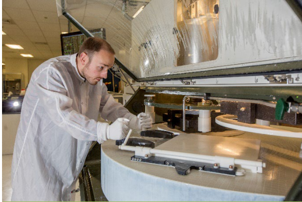
“Pizza peel” to safely remove optics under suspended load
