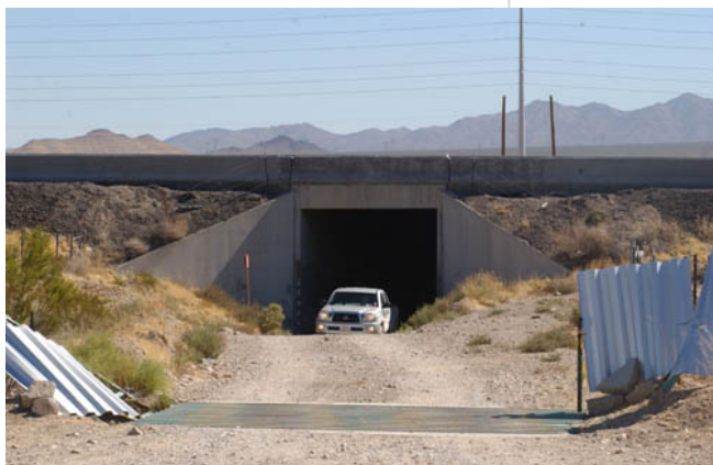
Two of the hazards on the DARPA Grand Challenge course. As vehicles go through the tunnel, they lose their GPS signal and must rely on other sensors. The narrow cattle gate requires the vehicle's sensors to be extremely accurate in sensing side obstacles and the center of the route.
