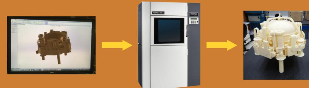
Digital printing and related technologies enable rapid iterations from concept to hardware prototype and even production.
