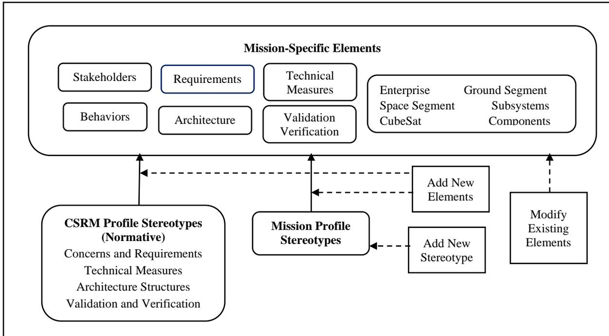
**The Mission CSRM is founded on the normative CSRM Profile Stereotypes with the addition of Mission Specific Stereotypes. The user can add new stereotypes, add new elements, and modify existing elements.**
