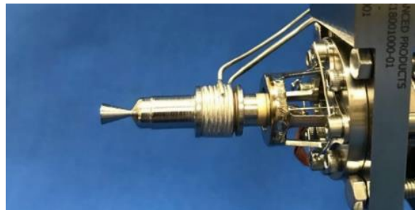
Figure 4.7: Rubicon 0.1N ASCENT thruster. Credit: NASA MSFC.
