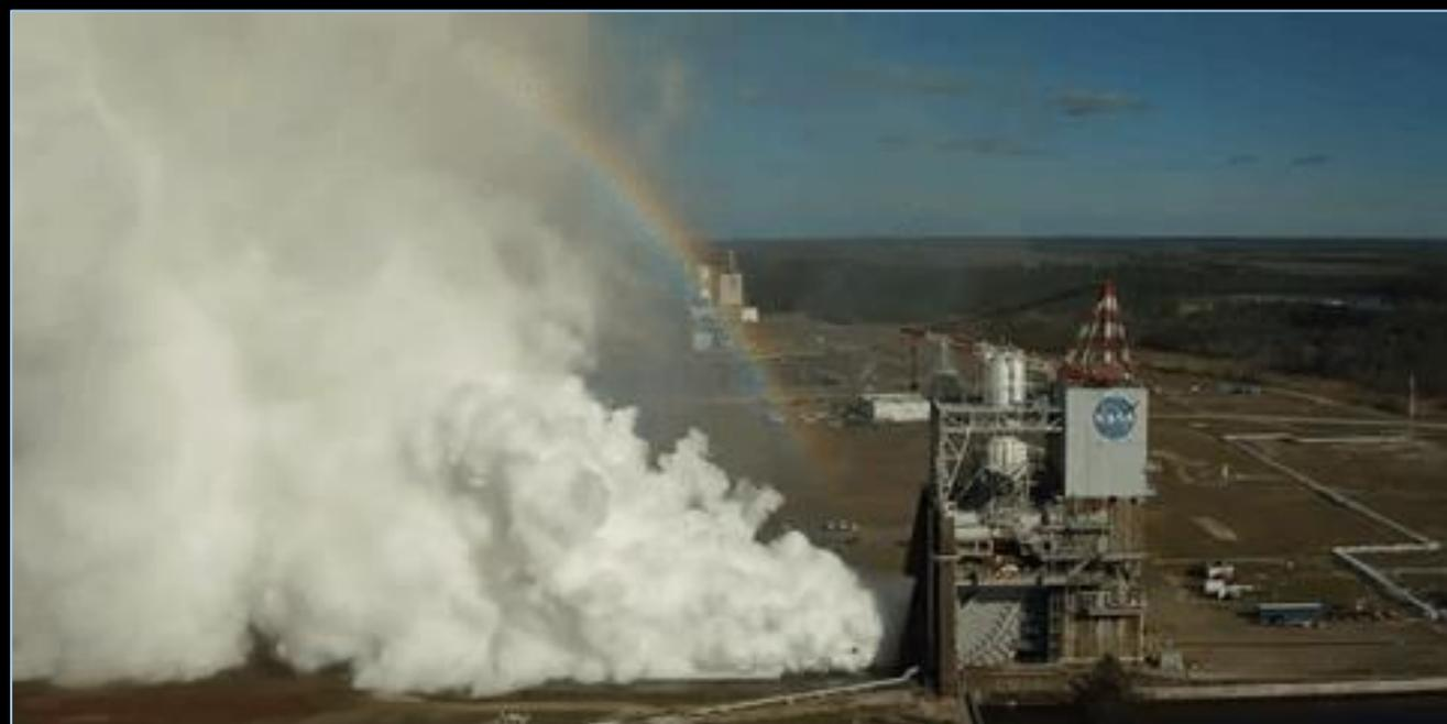
**RS-25 Rocket Engine Testing**
