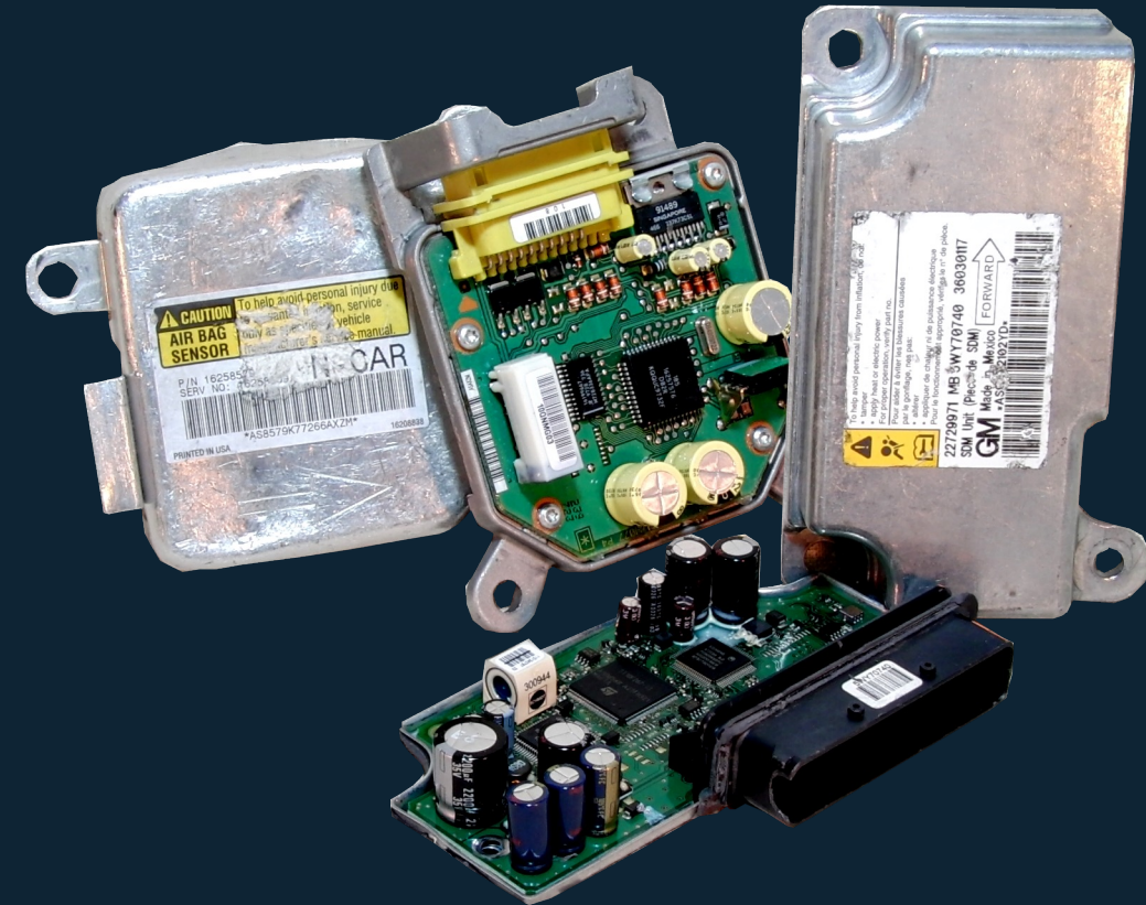
Event Data Recorder with some ECU's. Img src: https://crashdatagroup.com/pages/edr-explained
