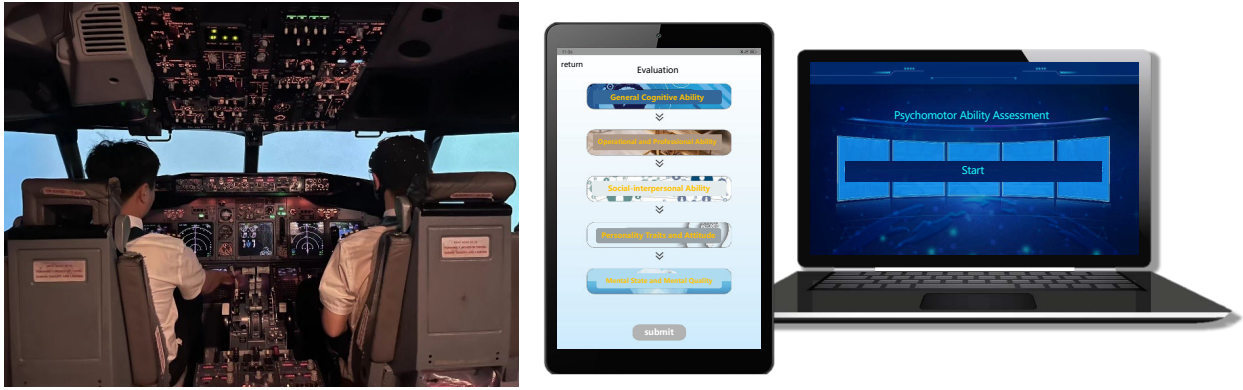
Figure 1. Apparatus (The tablet in the middle is used to assess pilots' general cognitive ability and social-interpersonal ability, while the computer on the right is primarily employed to evaluate pilots' psychomotor abilities.)
