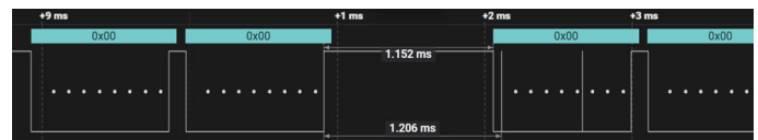
Figure 8. Valid MID 0x00, Valid Checksum 0x00, Surpassing Valid Inter-Frame Gap (BAT) < 1.255 ms
