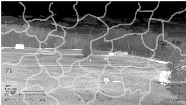
Figure 2.1-1: Conceptual Distribution of Multiple Isoplanatic Patches Across the Field of View.
