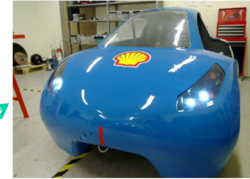
Figure 23: Near- and far front lights working correctly.
