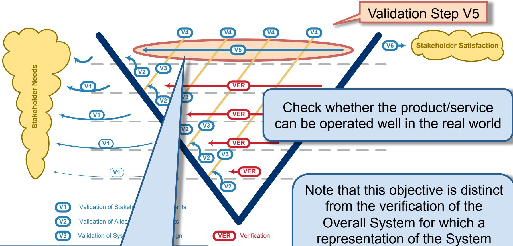
V5 is performed by bringing the integrated Overall System into its System Environment
