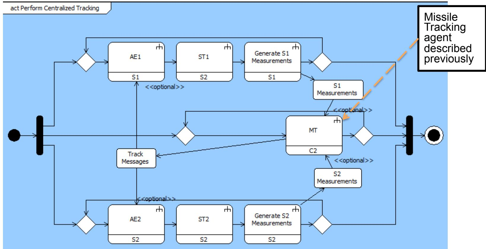
Sn = Sensor n, MT = Missile Tracking, AEn = Assessment and Evaluation n, STn = Sensor Tasking n, C2 = Command and Control
