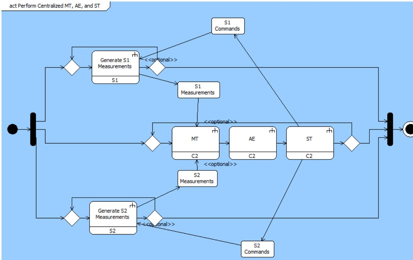
S1 = Sensor 1, S2 = Sensor 2, MT = Missile Tracking, AE = Assessment and Evaluation, ST = Sensor Tasking, C2 = Command and Control
