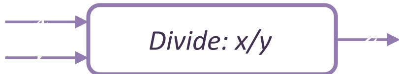
$$\mathcal{C}_1 : \left\{ \begin{array}{l} \text{variables: } \left\{ \begin{array}{l} \text{inputs: } x, y \\ \text{outputs: } z \end{array} \right. \\ \text{types: } x, y, z \in \mathbb{R} \\ \text{assumptions: } y \neq 0 \\ \text{guarantees: } z = x/y \end{array} \right.$$
