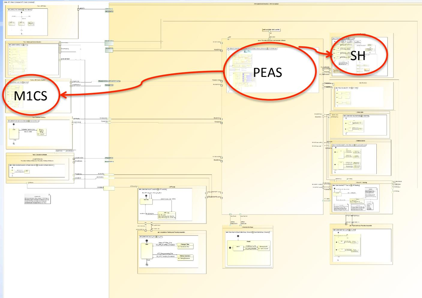
Communication between state machine specified components over ports
