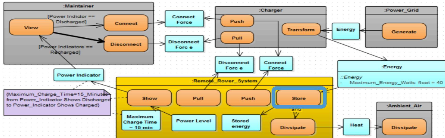
The **Remote\_Rover\_System** shall **Store Stored\_Energy** with the **Maximum\_Energy\_Watts=40** while in **Being Maintained** state.
