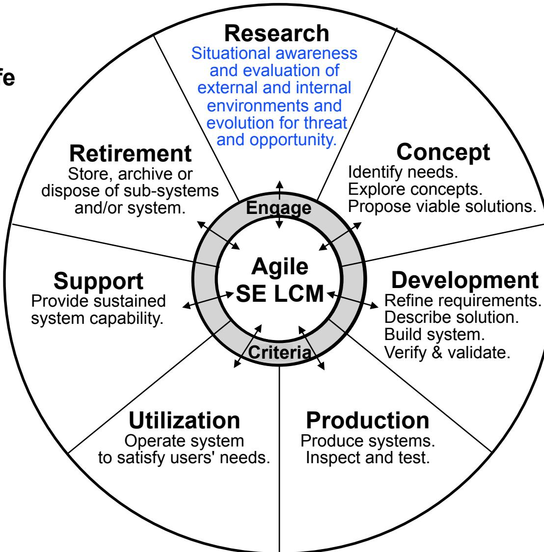
Seven asynchronously-invoked stages are engaged repetitively and simultaneously when engagement criteria are met
