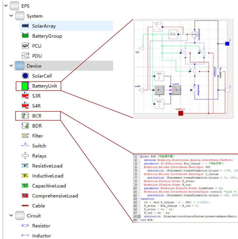
In *System Level 0*, high-level systems of spacecraft are built. There are three types of model in this level: *power supply system model*, *distribution system model* and *load system model*. The parameters of these models include *voltage*, *current*, *power*, etc.
