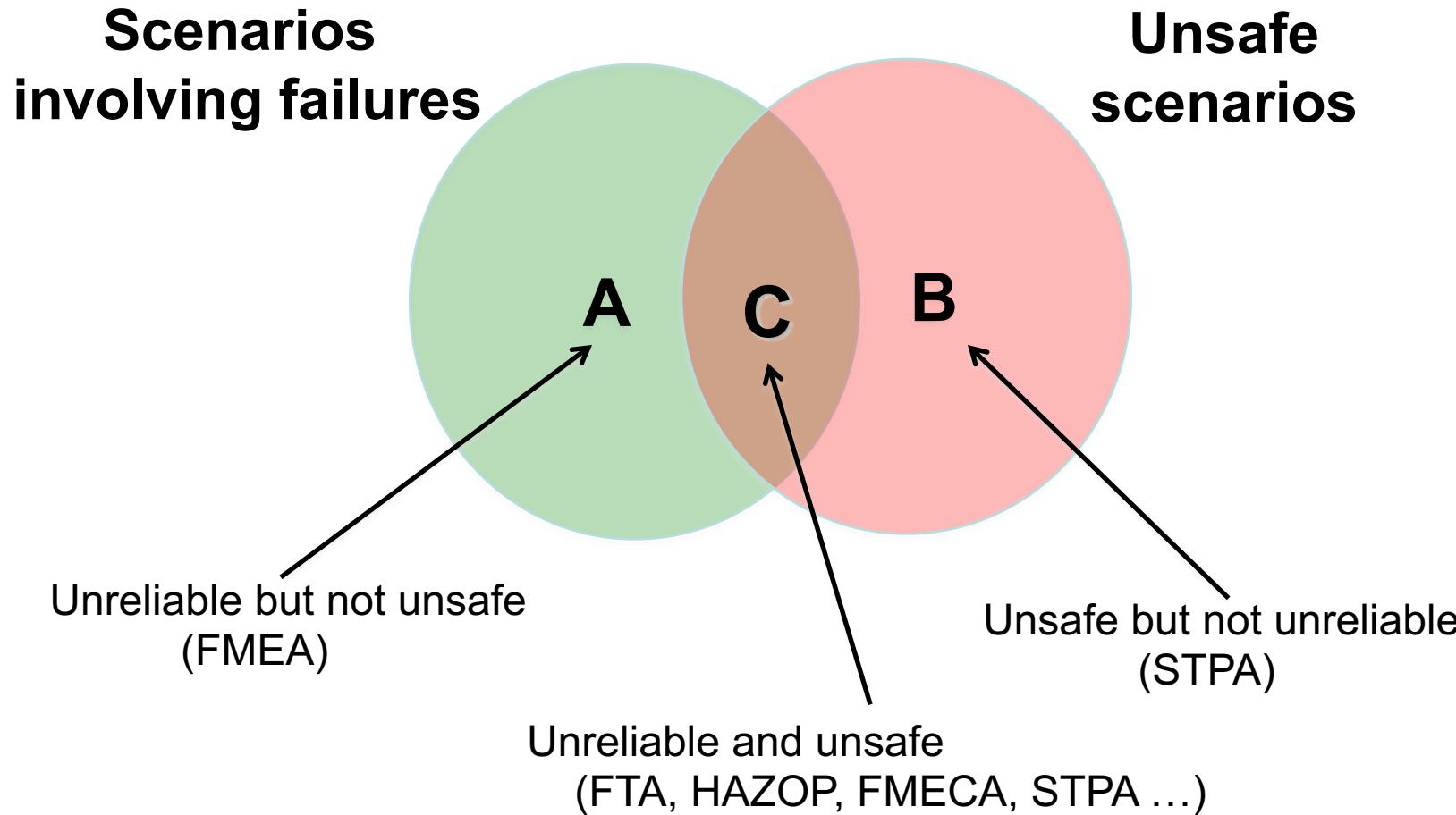
**Preventing Component or Functional Failures is Not Enough**
