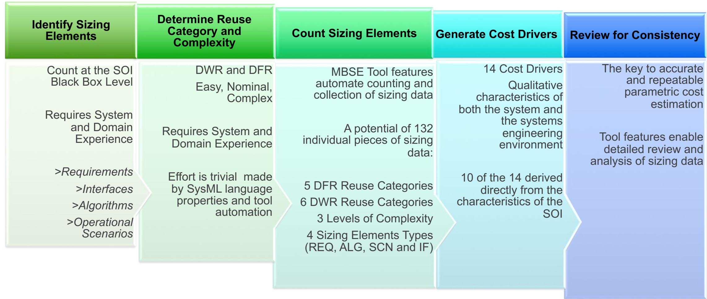
The Linchpin is identifying cost model inputs directly from the SysML attributes, as models are developed
