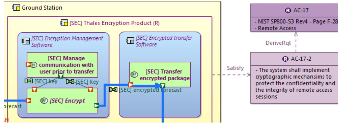
The assessment of how and how well the architecture elements contribute to the satisfaction of cybersecurity requirements, allow co-engineering teams to gain confidence on the solution architecture
