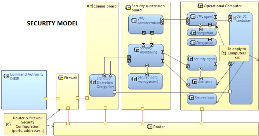
Cybersecurity-dedicated view - the Operational Computer physical component is a “representative” of several physical components in the system model. A set of behavioral components represent the cybersecurity-specific features that the latter shall implement.
