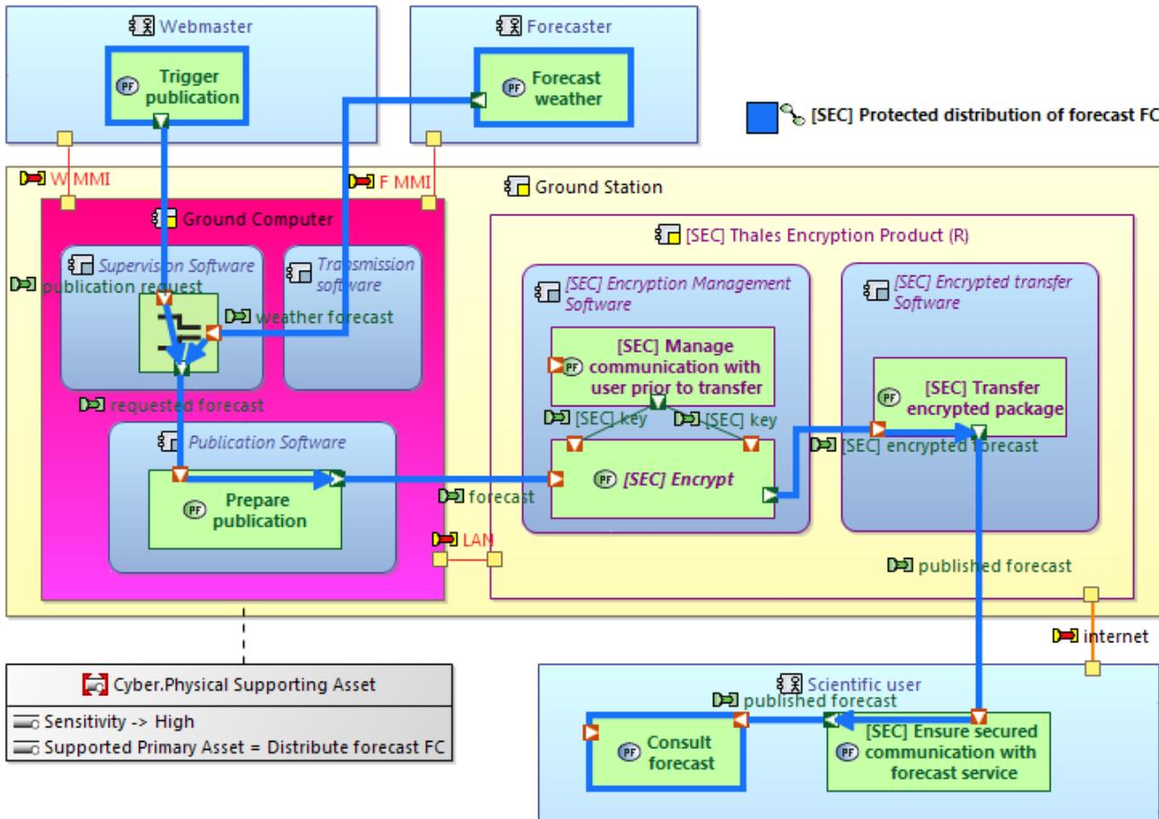
The definition of the architecture includes the identification of the **supporting assets** to be protected, and the functions and components that will implement the **security controls**.
