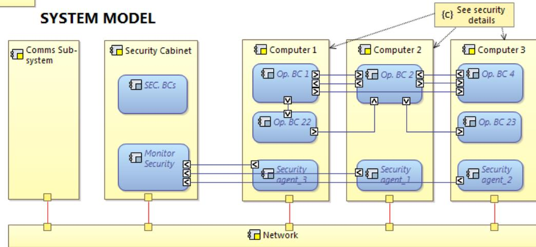
System-dedicated view – only those cybersecurity aspects impacting the system-level evaluations (sizing, interfaces,...) are represented, irrelevant details are omitted (e.g. Security Cabinet)
