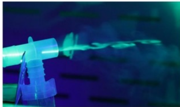
Carboxyl Polystyrene Blue Particles, 5% w/v, 0.21 \mu\text{m} , 1 mL. Spherotech CPB-02-10, Green laser (500-540nm <5mW)
