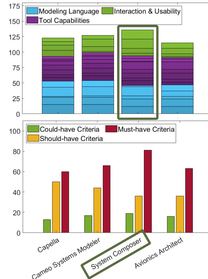
***System Composer* identified as most suitable tool for model-based, knowledge-driven systems architecting for presented application case.**
