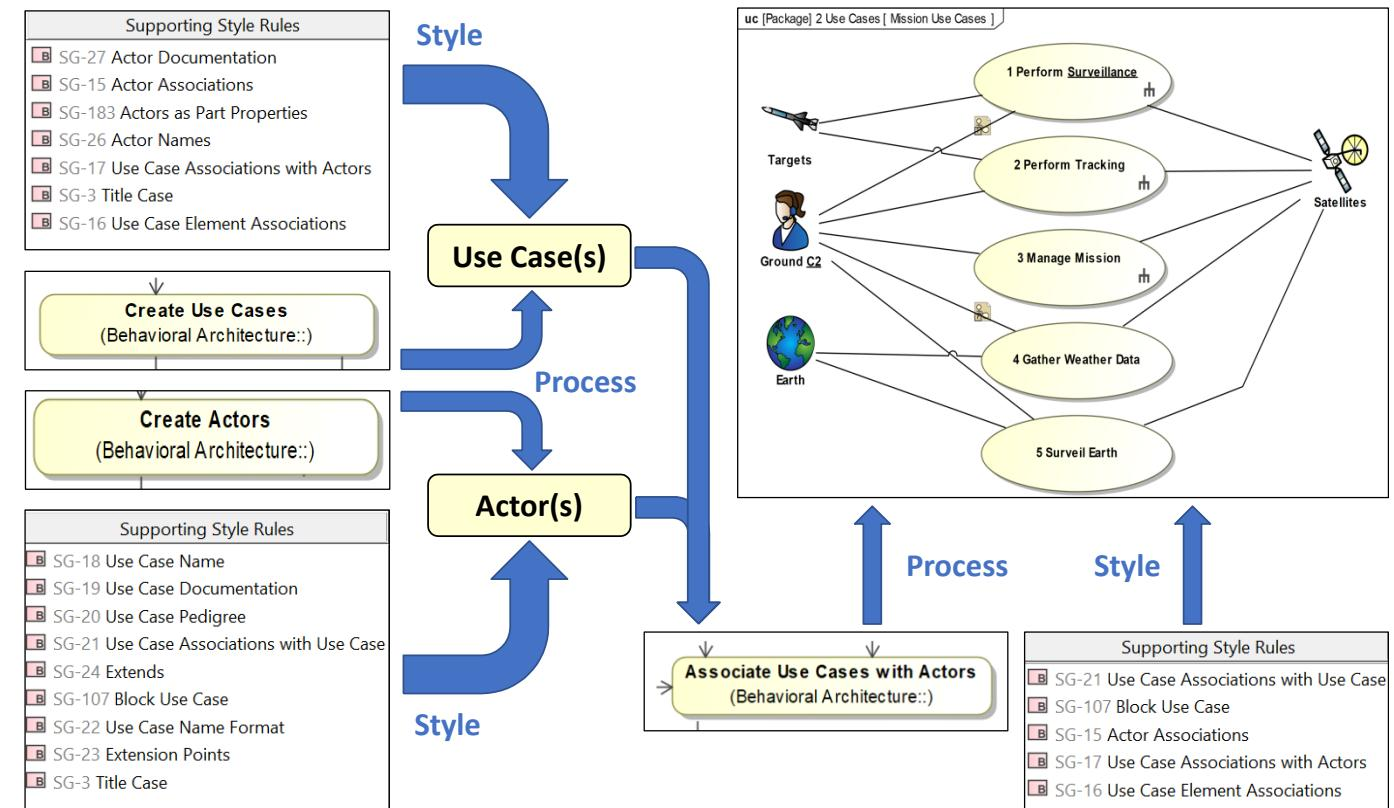
System operational context defined through use case development to enable functional architecting
