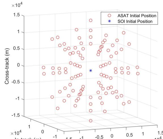
104 initial configurations (initial ASAT/SOI engagement geometry)
