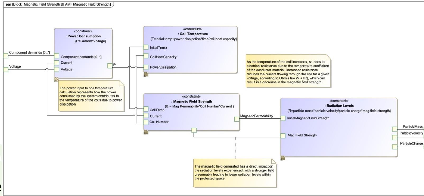
Parametric diagrams show how parameters are linked within the system and how simulations are used to validate system performance against requirements.
