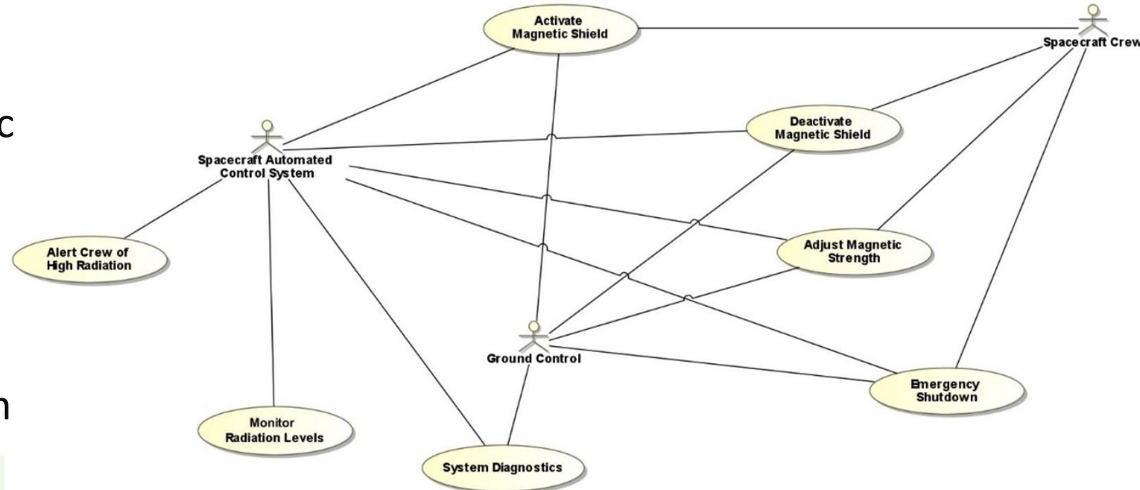
Use case diagrams show how different users (like astronauts and ground control personnel) will interact with the system, highlighting the system's functionality and user interfaces.
