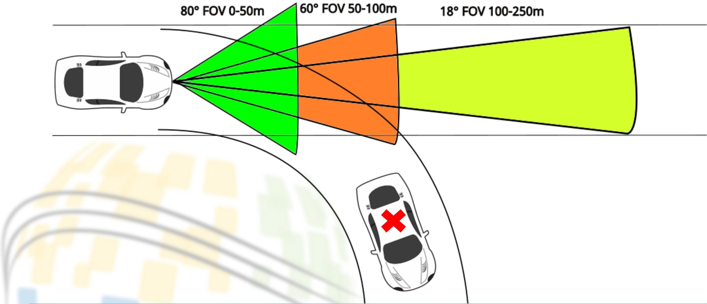
**Loss of Signal because of curve and the FOV of sensor**
