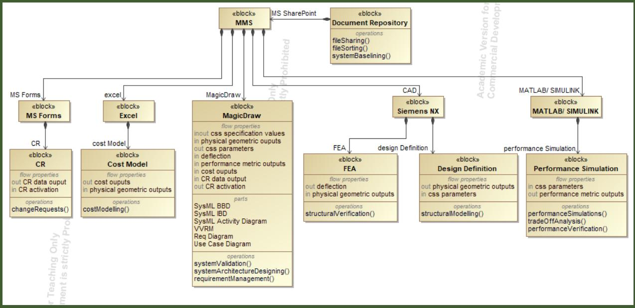
Specific model parameters tightly coupled via a tailored Internal Block Diagram (IBD); flow properties for model calls; embedded Parametric Diagrams and Constraint Blocks for compiled model code.
